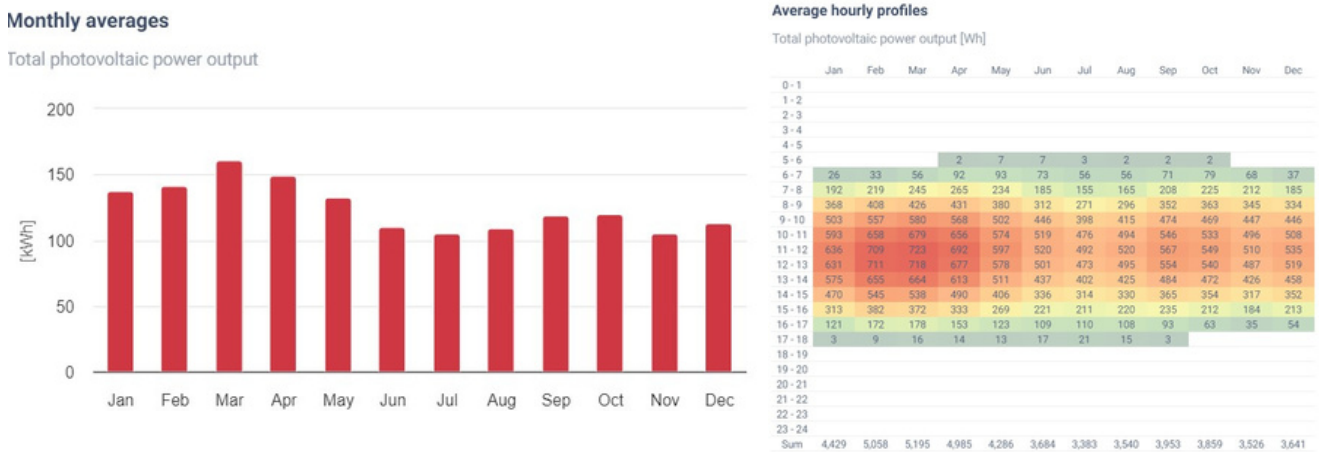
Fig 6: Monthly and hourly averages of solar radiation graph from Global Solar Atlas
